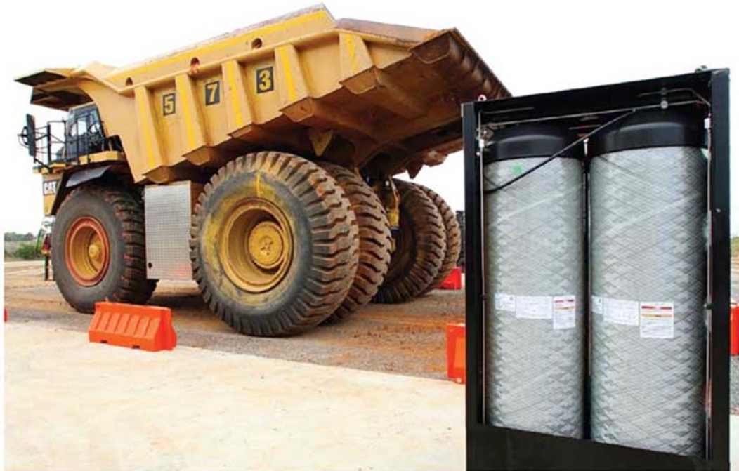
Figure 3-3: HDCNG Storage Tanks on a Mine Haul Truck
